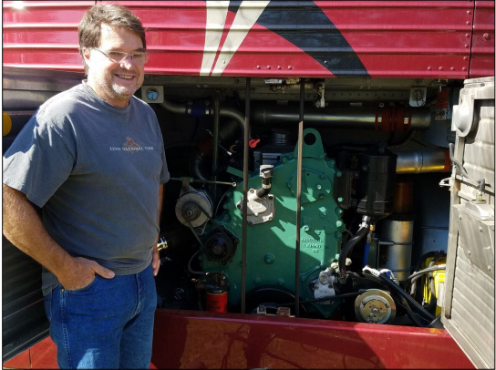
Laurier Poirier shows off the immaculate installation of a DD Series 50 in his MC-7.
